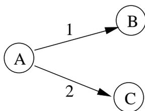
**Figure 3.5** Example illustrating the lack of kernel support for specifying the channel to use to reach a neighbor.
