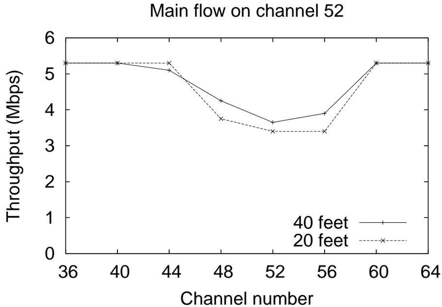
**Figure 3.1** Throughput with the presence of interference on each lower and middle band channel, nodes are separated by a distance of 20 ft and 40 ft. Throughput with no interference is at 5.3 Mbps.
