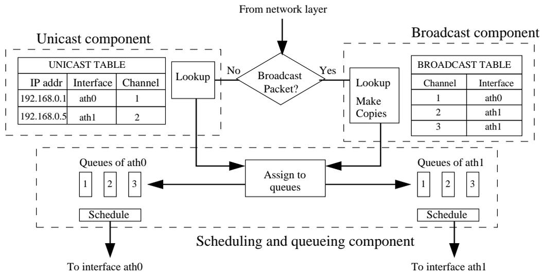
**Figure 4.2** Components of channel abstraction module: Tables are filled with the assumption that there are two interfaces “ath0” and “ath1,” and three channels.
