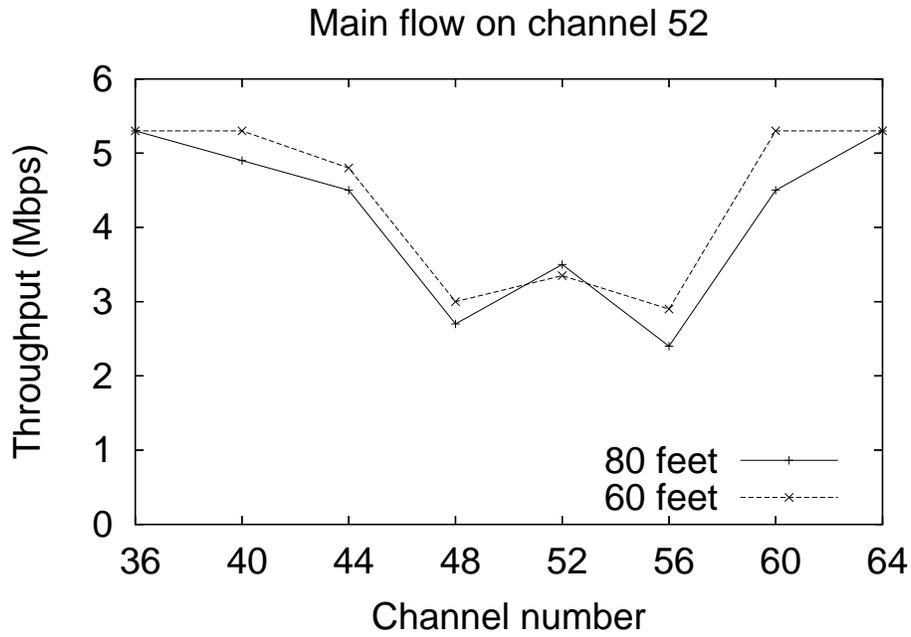
**Figure 3.2** Throughput with the presence of interference on each lower and middle band channel, nodes are separated by a distance of 60 ft and 80 ft. Throughput with no interference is at 5.3 Mbps.
