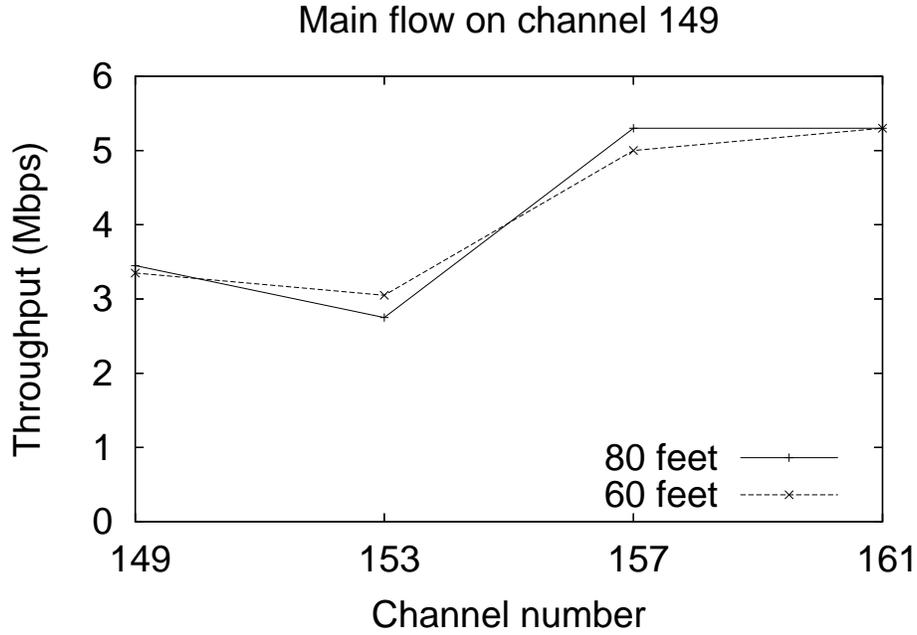
**Figure 3.4** Throughput with the presence of interference on each upper band channel, nodes are separated by a distance of 60 ft and 80 ft. Throughput with no interference is at 5.3 Mbps.
