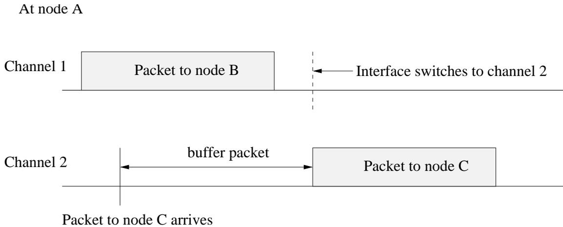
**Figure 3.6** Example illustrating support required for queuing and switching.
