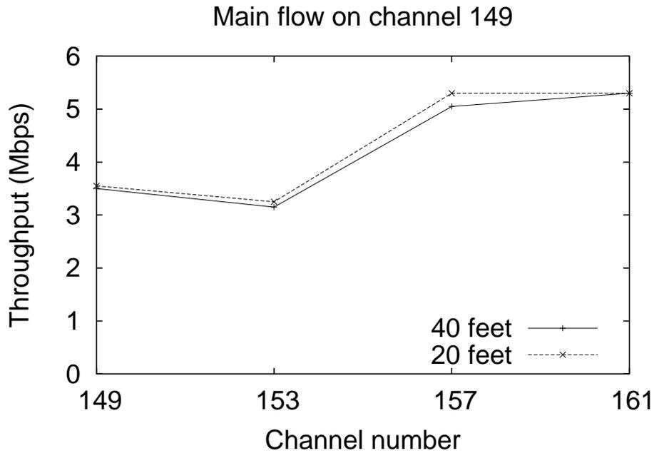
**Figure 3.3** Throughput with the presence of interference on each upper band channel, nodes are separated by a distance of 20 ft and 40 ft. Throughput with no interference is at 5.3 Mbps.
